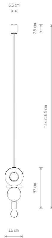
DROPS WOOD E plywood, painted steel
